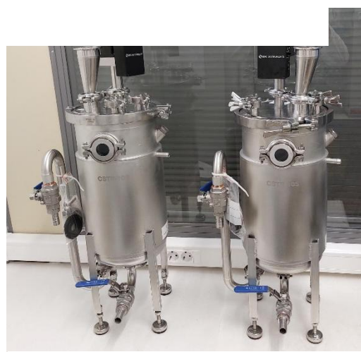
Figure 7. 10L-CSTR used by AINIA in Semi-continuous AD assays.
