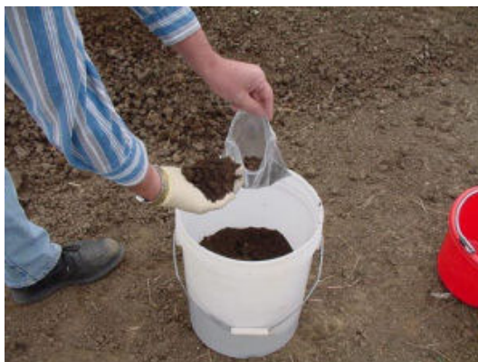
Figure 2. Mixing of the collected solid manure in a large container (bucket) to obtain a final subsample stored in a smaller sealed container (plastic bag)
